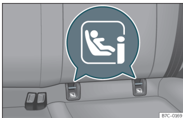
Fig. 32 ISOFIX/i-Size securing rings.
